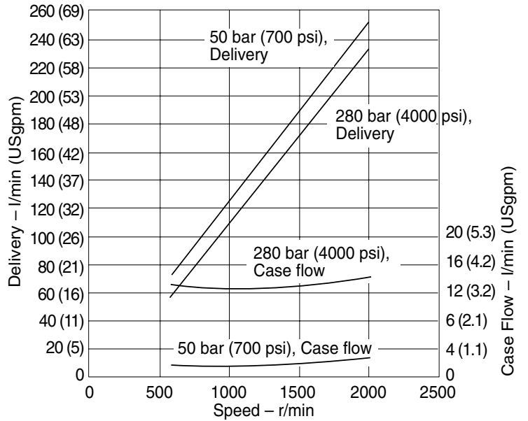
Delivery and Case Flow Versus Speed @ 93°C (200°F), full flow and 1.0 bar absolute (0 psi) gauge Inlet
