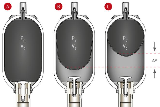
$V_0$  = Total gas volume of the accumulator
